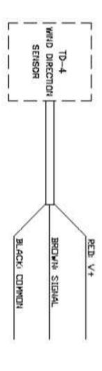
TYPICAL RANGE 0-360' Mechanical, 5k OHM: 0-355' Elect., 1DK OHM: 0-357' Elect.
