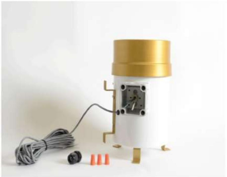
**Be Sure to remove Debris screen from top of collector during snow or icing conditions.**
