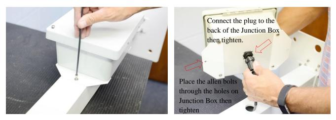
• Remove the (2) allen bolts above and below the 1½" hole. This is the connector that will hook up to the Junction Box
