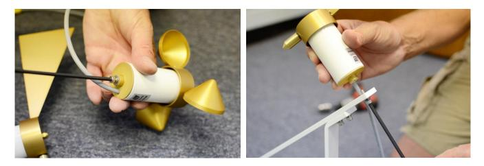
• Remove the allen bolts on the bottom of each Wind Sensor (1) each the place them at each end on the "V-Shape" bracket. Connect and tighten allen bolts.
