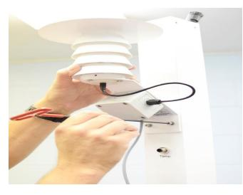
Remove (2) allen bolts on the front of the Mast to mount the Temperature & Humidity Sensor. Align holes and insert allen bolts. Connect and tighten sensor to Mast.
