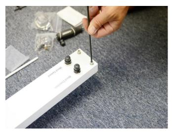
Remove (2) allen bolts on the end of the cross arm label "Wind Speed/Wind Direction".
